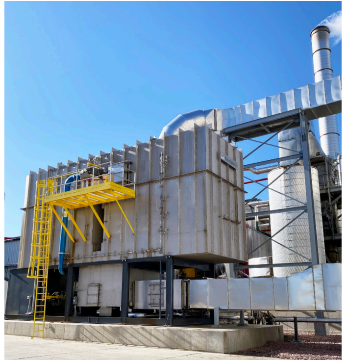
Oxi.X RC regenerative thermal oxidizer.
