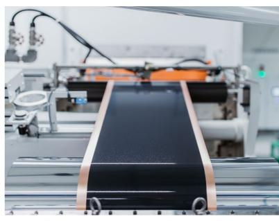
Shift work: The drying process follows shortly after electrode coating.
