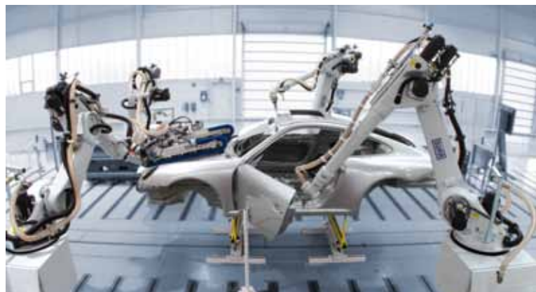
Robotic cleaning installation with sword brushes and suction and blowing unit
