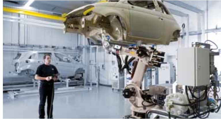
Sealing/gluing section of the Ecopaint Test Center
