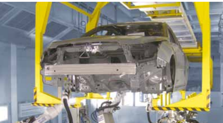
Ecopaint Sealing station for seam sealing and underbody protection
