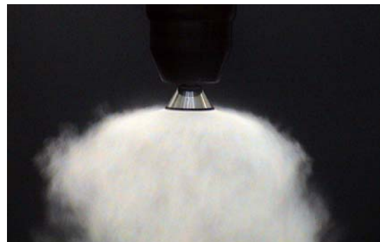
Shaping air setting for exterior painting
