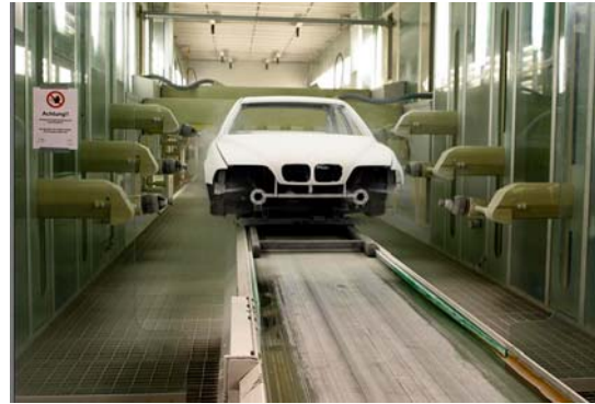
EcoBell Powder F Atomiser during painting exterior painting with Ecopaint side machines
