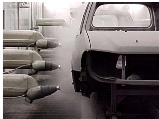
EcoBell Powder F atomizer during painting exterior painting with Ecopaint side machines
