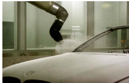
EcoBell2 Powder atomiser during exterior painting
