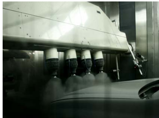
EcoBell Powder F2 atomiser during painting exterior painting with Ecopaint roof machine
