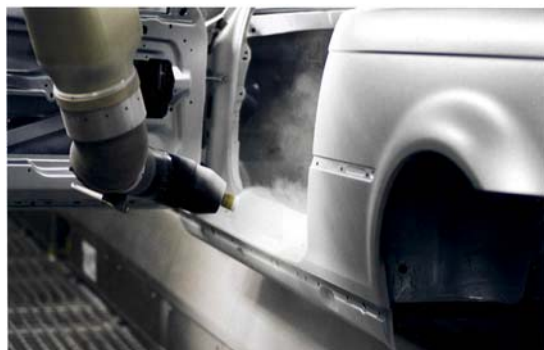
EcoBell2 Powder atomiser painting interior (cut-in)
