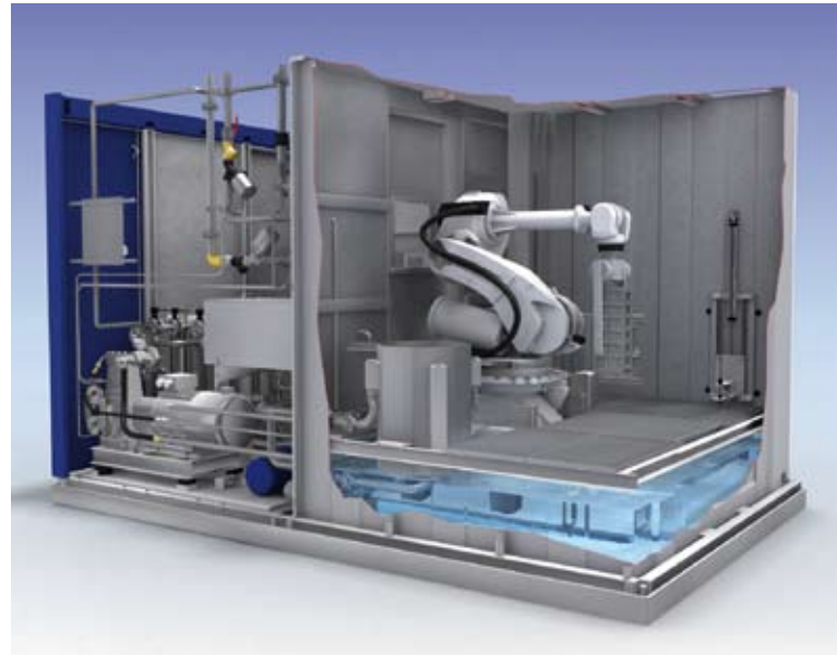
Treatment module with integrated 6-axis robot
