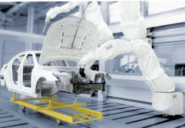
Robots on travel rails arranged one above the other shorten the booth length
