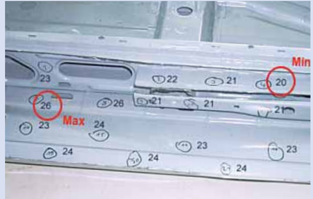
Cavity film thickness measurements after RoDip rotation
