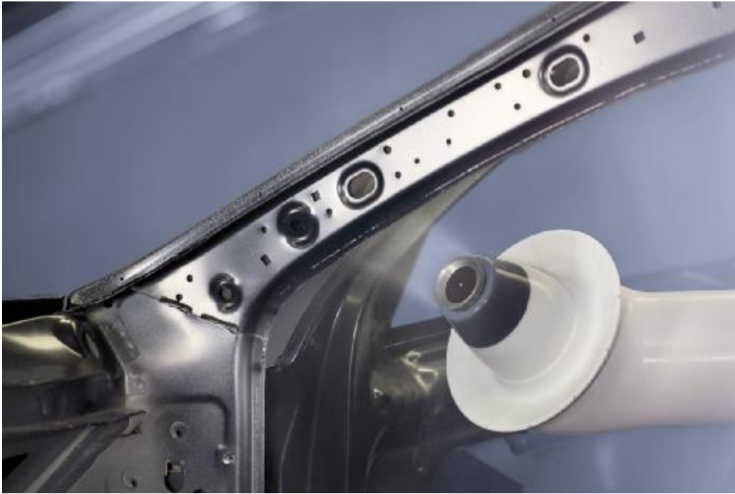
EcoBell3 interior painting: With high-speed rotating atomizer and direct charging.
