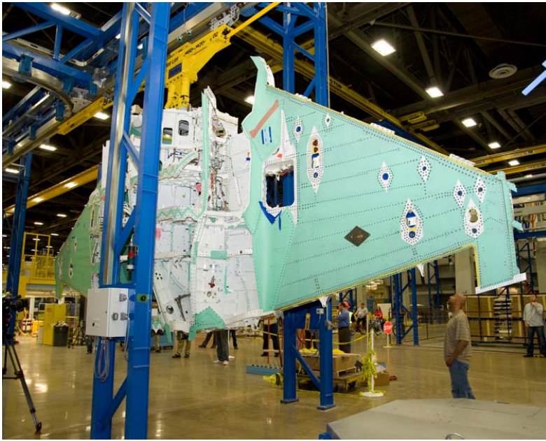
Photo 2: FASTplant® heavy duty modules for aircraft manufacture in operation at Lockheed Martin.
