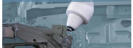
» EcoBell3 Cx for bumper painting and for combined zones with interior and exterior painting
