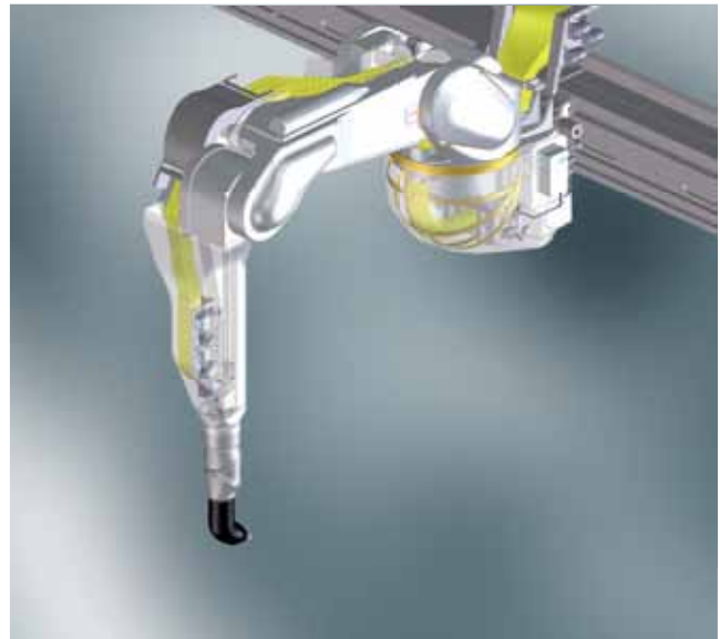
» Central cable routing through the robot axes
