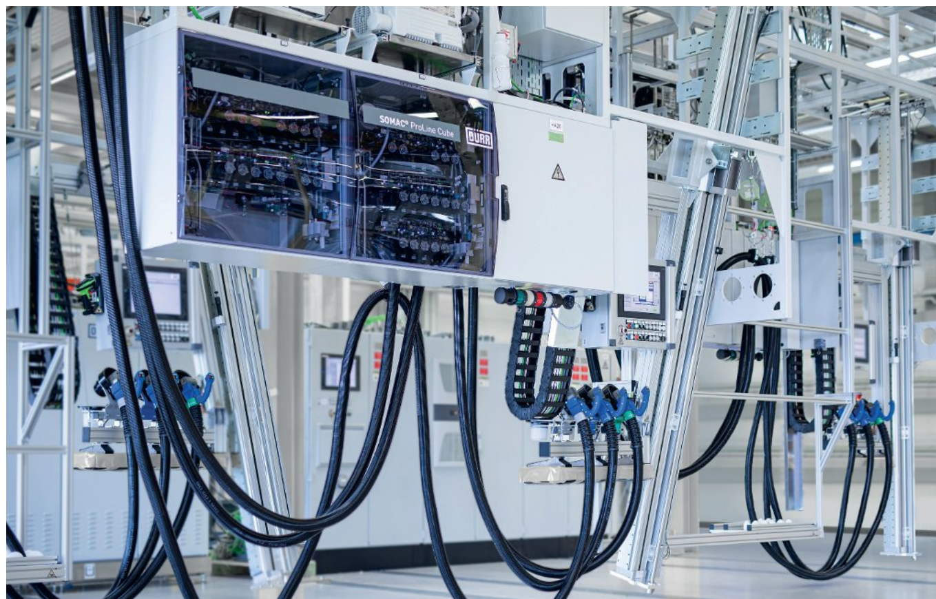
Combined filling of all media types with one ProLine Cube filling machine
