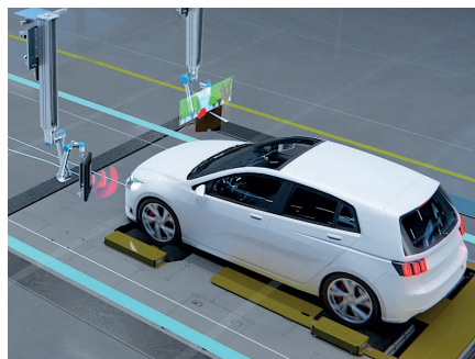
Fig. 2: x-around, dynamic radar object positioning
