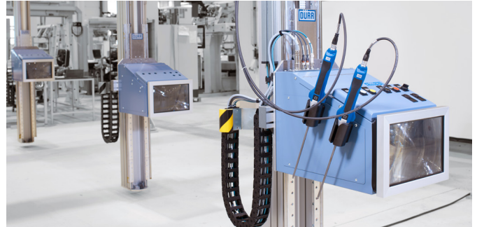
Headlamp adjustment x-light with setting tool Smart Ergo Drive
