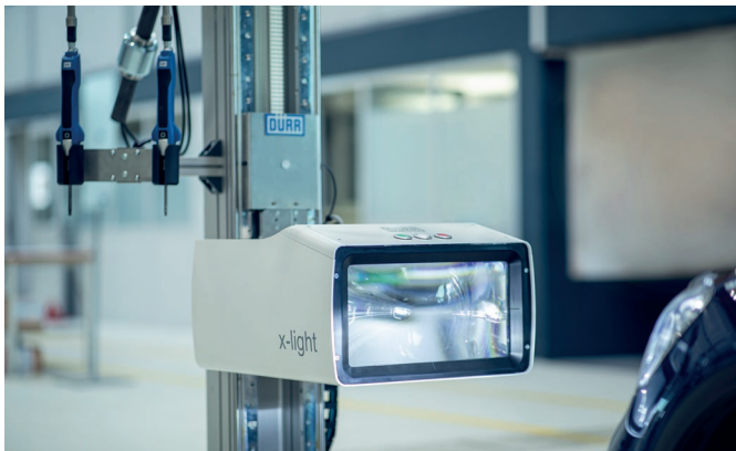
Light measuring device with Smart Ergo Drive
