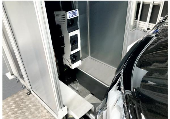
Measuring sensor x-3Dsurface
