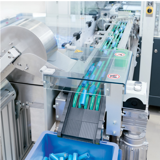
Cell feeding with bunker solution.
