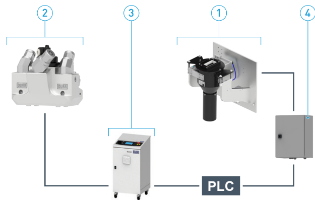
1 EcoPaintJet Cleaner, 2 EcoPaintJet, 3 Application controller, 4 Pneumatic control unit, PLC Master painting process control system,
