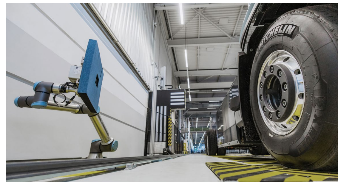
Collaborative robot with side-radar-calibrated target
