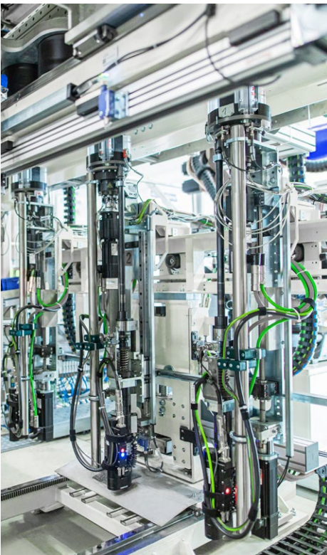
x-gun, the bolting system for direct bolting combined with the NC driven bolting station x-bolt
